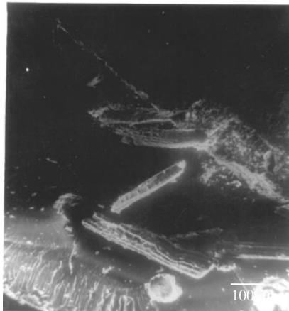
Figure 5 SEM for the fractured banana fiber composite on tensile loading (70X)
